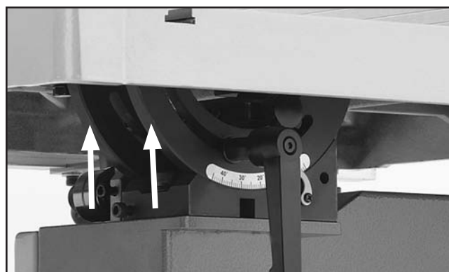
Figure 95. Trunnion lubrication location (G0514X2/G0514X2B/G0514X3).
