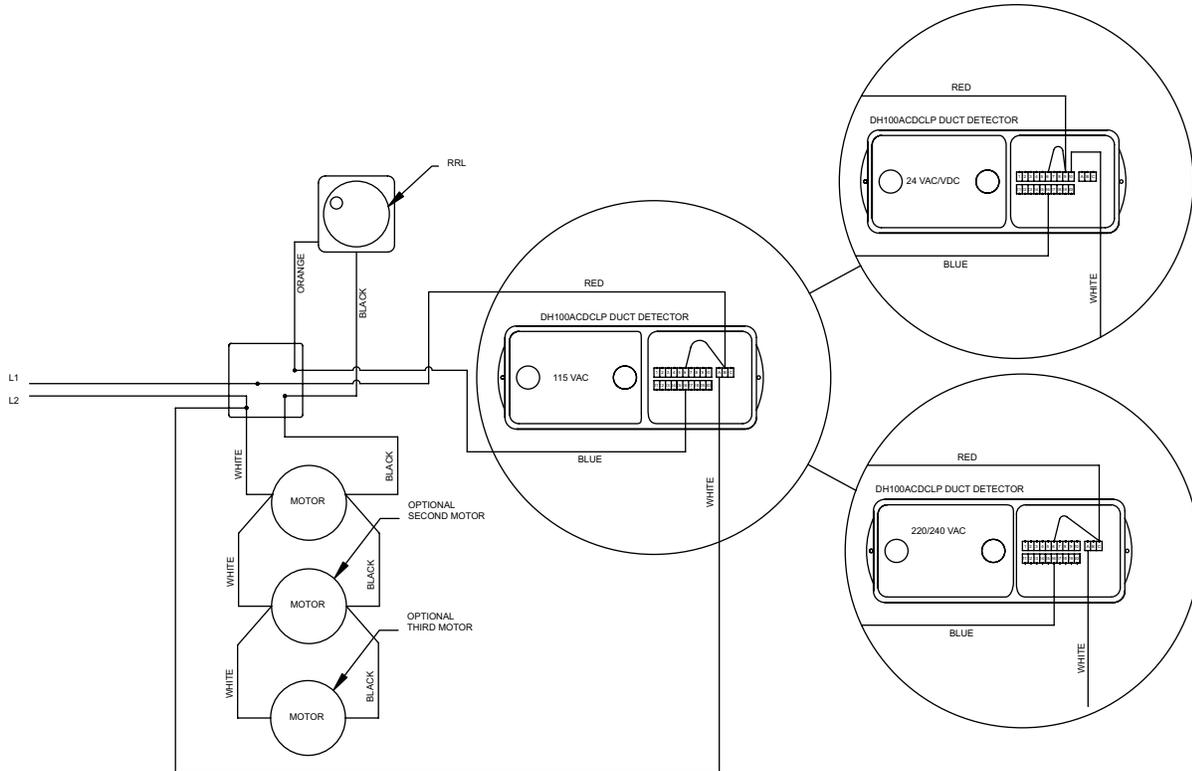
1. CONDUIT RUNS WHICH EXCEED 72" MUST HAVE GREEN GROUND WIRE.
