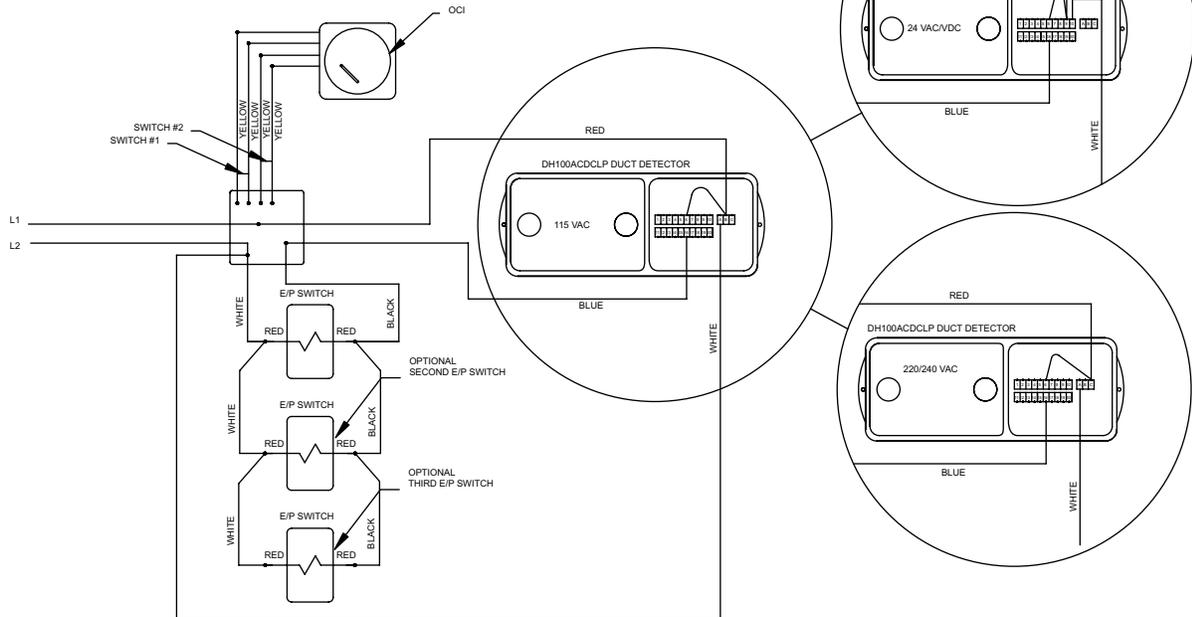
1. CONDUIT RUNS WHICH EXCEED 72" MUST HAVE GREEN GROUND WIRE.
