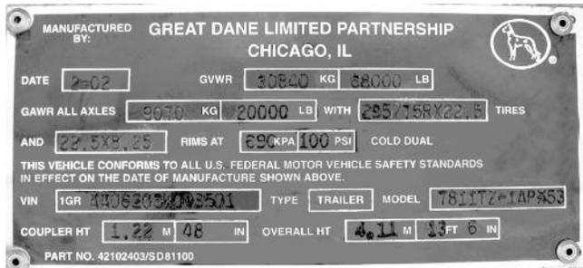
The GAWR and tire information shown on the vehicle certification plate was applicable at the time the trailer was manufactured. If the tires or other components of the running gear have been changed or altered since the trailer was manufactured, the GAWR may have changed. This should be checked with Great Dane Trailers Customer Service Department.
