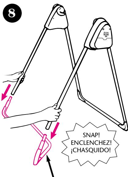
**CHECK** that all tubes are securely attached. Button **MUST** snap through hole. **CHECK** that the parts of the frame are assembled in the positions shown.
