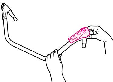
Place feet with the text "FRONT BOTTOM" onto the front tube as shown. The text "FRONT BOTTOM" should face floor.
