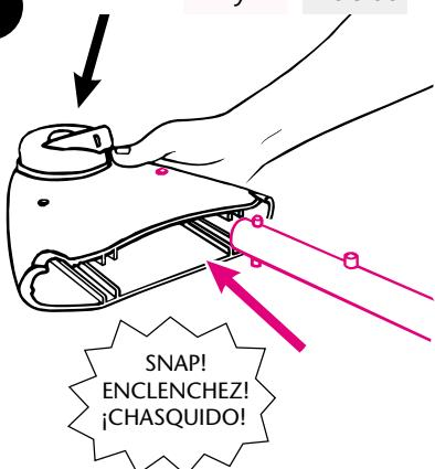
The double buttons must fit into the channels inside the housings.
