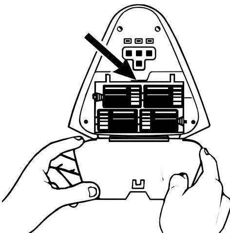
**With baby out of swing,** open the battery compartment lid by inserting a coin (penny, nickel or dime) into the coin slot. Insert four "D"-LR20 (1.5V) cell batteries.
