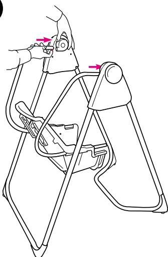
**CHECK** that hanger tubes are secure in brackets by pulling firmly on them.
