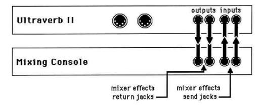
Generally, you'll want to insert the Ultraverb II into the mixing or PA console's stereo effects send/return connections. Set the Ultraverb II's Effect Mix control fully clockwise so that it passes only the processed signal; adjust the mixer's send levels for the proper Ultraverb II signal level (as indicated by the Clip/Signal LED), and use the mixer's return controls to set the desired blend of processed sound in relation to the overall mix.
