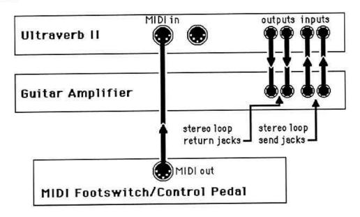
The Ultraverb II plugs into the stereo effects loop of a guitar amp. If the loop level is adjustable, it should be set to line level (not guitar level). If the loop is mono, plug the loop send into the Ultraverb II left/mono jack, and patch either Ultraverb II output into the loop return jack. Set the Ultraverb II's
