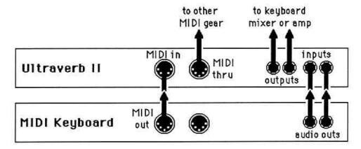
Patch the keyboard's audio outputs into the Ultraverb II's inputs, then send the Ultraverb II's outputs to a keyboard mixer or other amplification system. Patch the keyboard's MIDI out to the Ultraverb II's MIDI in; this allows the Ultraverb II to change patches as you change programs on the keyboard, as well as respond to keyboard parameters such as pressure, pitch bend, etc.
