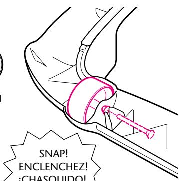
**CHECK** that wheel pins are held securely in place by plastic tabs.
