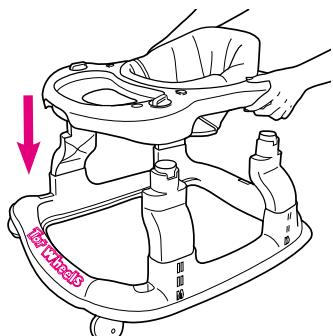
**WARNING** For the safety of your child, front of tray must go above front of base (which has "Tot Wheels" design and castors).
