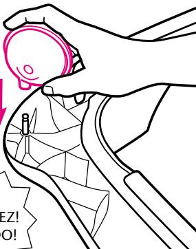
**CHECK** that castors are securely attached to base by pulling firmly on them.
