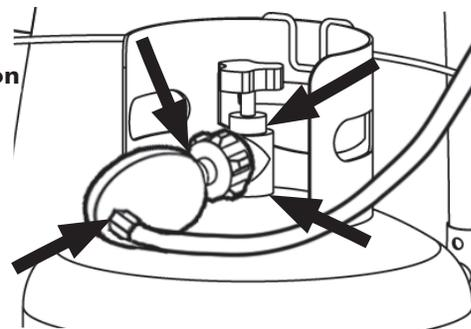
5. Check for leaks by brushing the soap solution on all gas valves, hose connections and fittings. (Shown by the heavy arrows in Fig. 2 & 3) Make sure you generously brush the locations with the soap solution, completely surrounding the connections and fittings.
