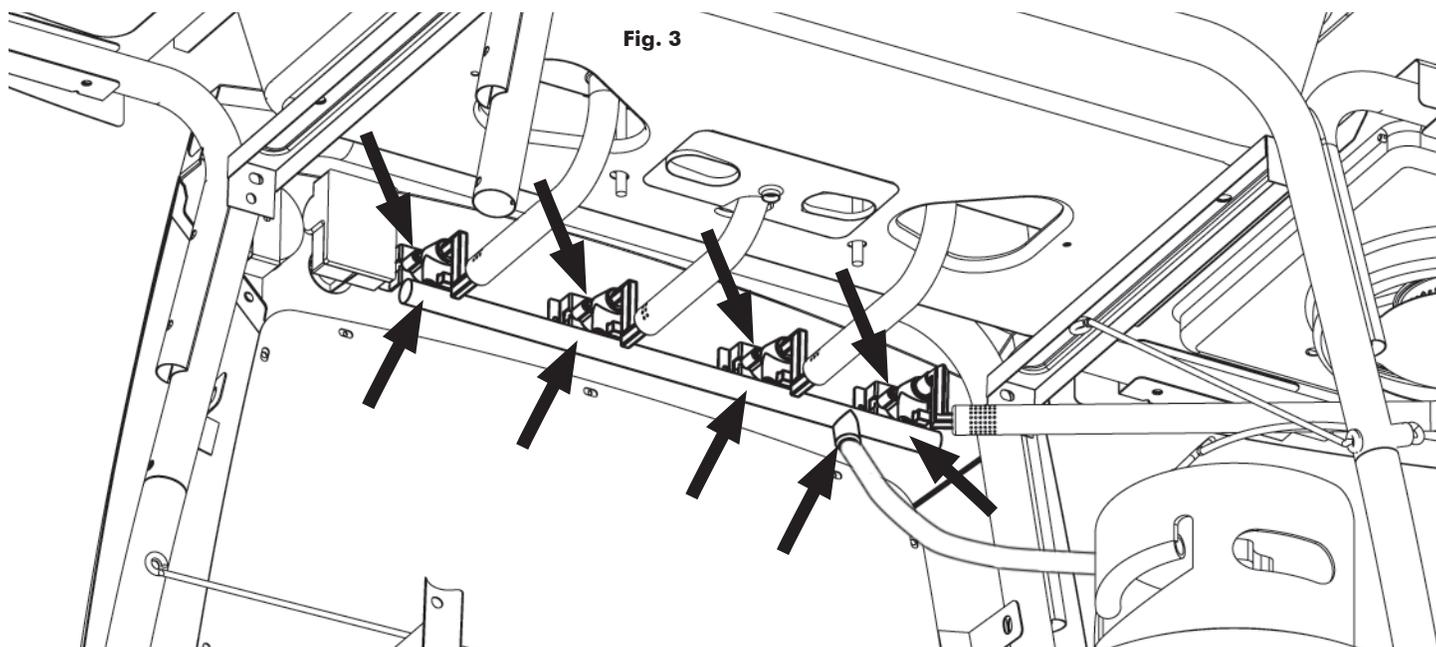
6. If “growing” bubbles appear on any of the connection points, you have detected a gas leak. Immediately close the LP Gas Cylinder valve by turning handle clockwise
