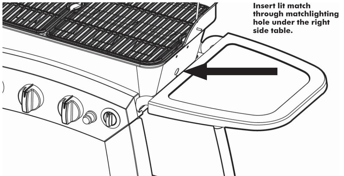
If any or all Burners fail to light after three or four attempts following Steps 3-4, turn all Control Knobs to the "Off" position and close the LP Gas Cylinder valve to dissipate any accumulated gas. Wait five minutes; then repeat the lighting procedures.
