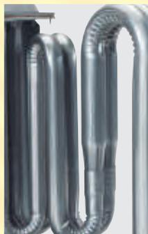
The award-winning design of the primary heat exchanger in the Goodman brand GMVC8 is unique. It's constructed from tubular aluminumized-steel and formed into a dual diameter configuration. Furthermore, the use of wrinkle-bend technology results in an extremely durable heat exchanger. A heat exchanger often is considered the essential component of any gas furnace. This combination offers one of the best levels of reliability, durability, and efficiency you'll find within the Goodman brand.
