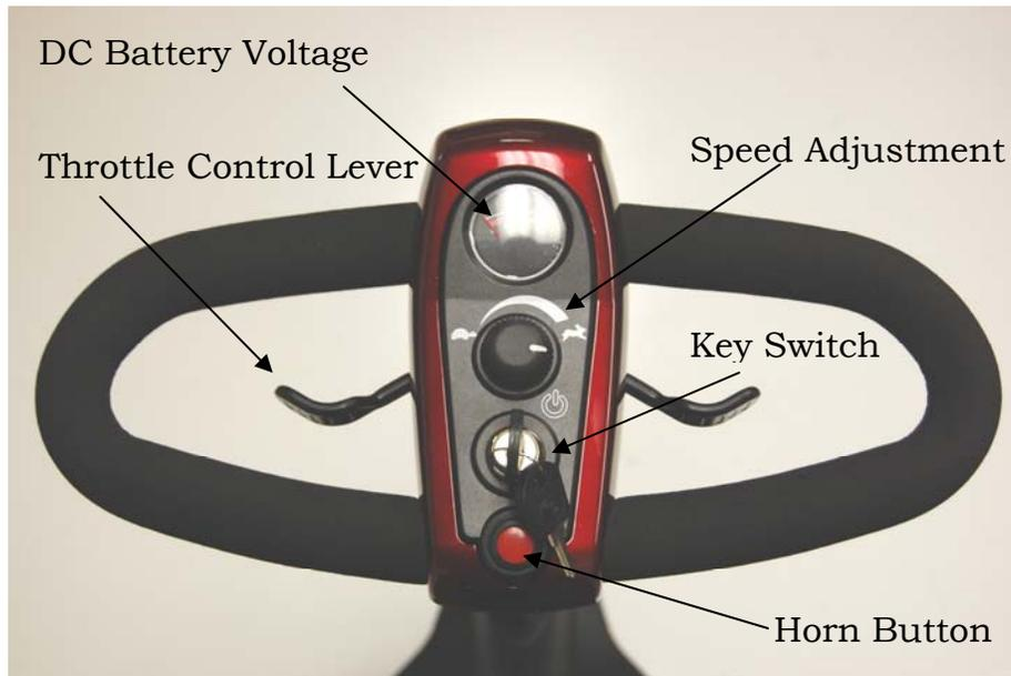
**Figure 5. Buzzaround XL™ Delta Tiller Control Panel**
