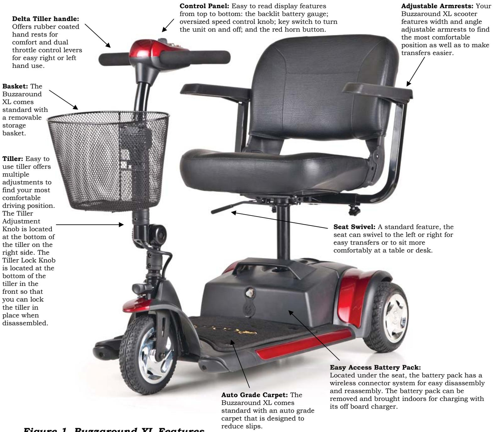
**Delta Tiller handle:** Offers rubber coated hand rests for comfort and dual throttle control levers for easy right or left hand use.
