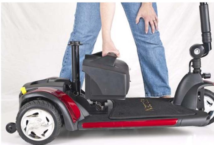
**Figure 22. Battery Pack Installation**
