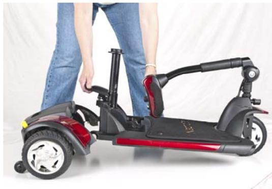
**Figure 18. Separating the Drivetrain and Frame**
