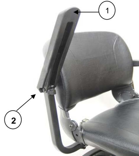
**Figure 7. Flip-up/Angle Adjustment**
