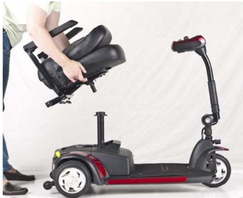
**Figure 15. Removing the Seat**
