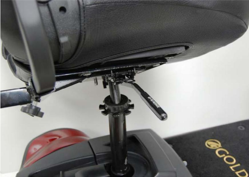
**Figure 24. Installing the Seat**
