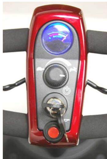
**Figure 14. Key Switch (On)**
