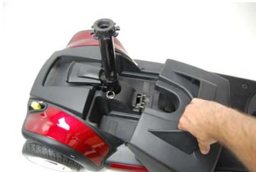
**Figure 16. Removing the Battery Pack**
