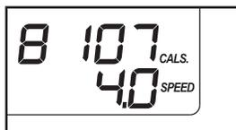
To reset the display, press the Stop button, remove the key, and then reinsert the key.
