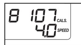
If you press one of the numbered speed buttons, the walking belt will gradually change speed until it reaches the selected speed setting.
