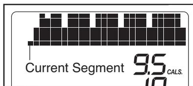
the profile represents the current segment of the workout. The height of the flashing segment indicates the speed setting for the current segment. At the end of each segment, a series of tones will sound and the next segment of the profile will begin to flash. If a different speed or incline setting is programmed for the next segment, the speed or incline setting will flash in the display to alert you.
