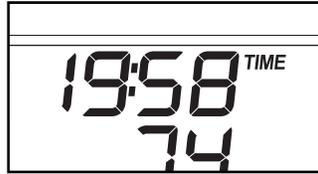
The lower half of the display will show your pedaling speed (revolutions per minute [RPM]) and the approximate number of calories you have burned. The display will change from one mode to the other every few seconds. The lower half of the display will also show your heart rate when you use the handgrip pulse sensor (see step 5).
