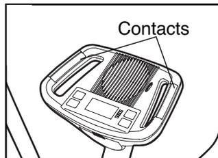
For the most accurate heart rate reading, continue to hold the handgrip pulse sensor for about 30 seconds. Note: If you continue to hold the handgrip pulse sensor, the display will show your heart rate for about 30 seconds. The display will then show your heart rate along with the other modes.
