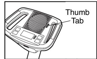
Rotate the thumb tab on the right side of the fan to adjust the angle of the fan.
