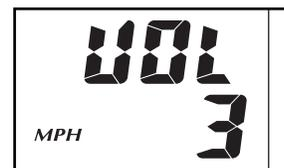
To change the unit of measurement, first press the Display button for a few seconds until the display is blank; then, release the Display button. Press the Fan button repeatedly to change the unit of measurement. You can also adjust the volume of the console tones at this time. Press the Magnetic Resistance increase and decrease buttons to select a volume level between 1 and 5. When you have selected the desired unit of measurement and volume level, press the Display button again.
