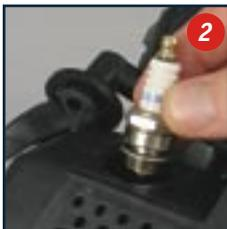
3. Clean and adjust the spark plug gap to 0.6 - 0.7mm. Replace any damaged or visibly worn plug with a worn plug with an equivalent spark plug, including NGK BM4A, CHAMPION CJ14, DENSO W14M-U10, BOSCH WS8E.
