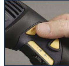
**CAUTION.** Any attempt to reverse the direction of rotation while the drill is turning is likely to permanently damage the switch.
