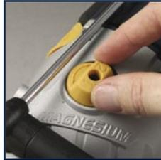
**NOTE.** Do not change gears when the drill motor is turning.
