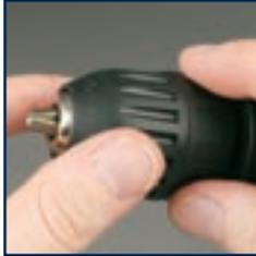
2. Ensure the drill bit is fully inserted, so that the chuck jaws grip the straight section of the bit.
