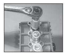
IMPORTANT! Care must be taken that glue does not get between the plunger pipe (16B) and centring sleeve (16C). The plunger pipe should not be strained by eccentric tightening of the tension screw or through damage to front surface of plunger, otherwise it is liable to fracture.
