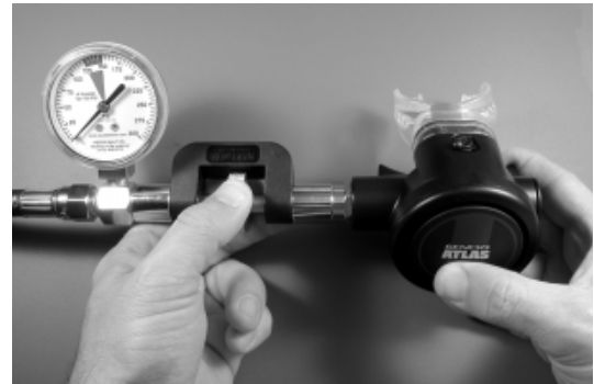
Fig. 20 - Inline Adjustment Tool w/ IP Gauge
