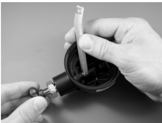
Fig. 8 – Disassembly of Poppet
