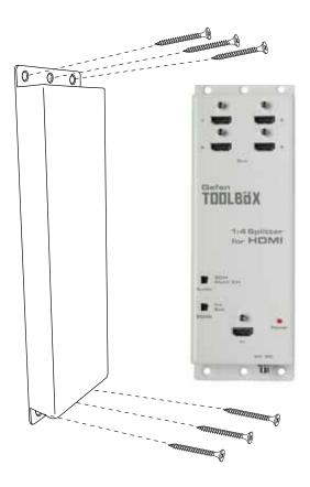
The GefenToolBox 1:4 Splitter for HDMI should be mounted vertically in a wall or cabinet with wood/drywall screws as shown in the diagram above. There should be an inch or two of clearance between the edges of the unit and any walls or vertical surfaces to allow for enough clearance for insertion and retraction of cables at the HDMI connectors.
