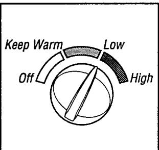
The Control Knob on the slow cooker offers Low and High temperature settings for cooking. The Keep Warm setting is for holding the prepared recipe at a perfect serving temperature.
