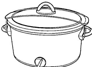
The **Lid Latch** secures the cover while moving, transporting, or storing the slow cooker. To use Lid Latch, place the white band into the groove located under one of the handles. Stretch the band to the other side of the slow cooker and secure it in the groove under the other handle.
