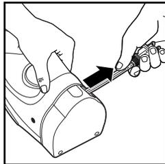
2. To store cord, press and hold Cord Release Button while guiding cord into storage area. **CAUTION:** Hold plug while retracting cord.
