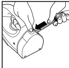
**CAUTION:** Hold plug while retracting cord. Do not let cord retract freely. Cord may jam on reel or loose cord may whip back and forth and could cause injury.
