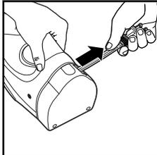
2. To store cord, press and hold the Cord Release Button while guiding the cord into the storage area.
