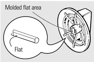
The knob stem is flat on one side (see illustration). Check the inside of the knob and find the molded flat area.
