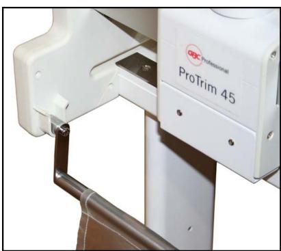
Attach the other waste curtain support bar to the stand of the trimmer with the bolts identified as "**B** "earlier in this manual.
