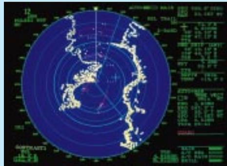
The Auto Plotter ARP-17 automatically tracks up to 20 targets acquired manually or automatically, presents target data, and triggers a collision alarm for the target on a collision course.
