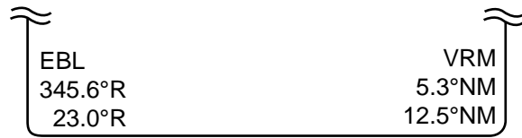
Figure 2-7 Display bottom, showing location of EBL and VRM readouts
