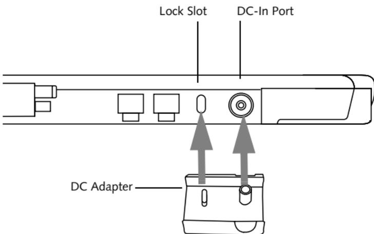
**Figure 1. Attaching the DC Adapter**
