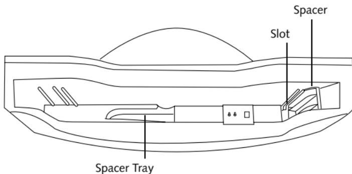
**Figure 2. Inside the Charge-Only Cradle**
