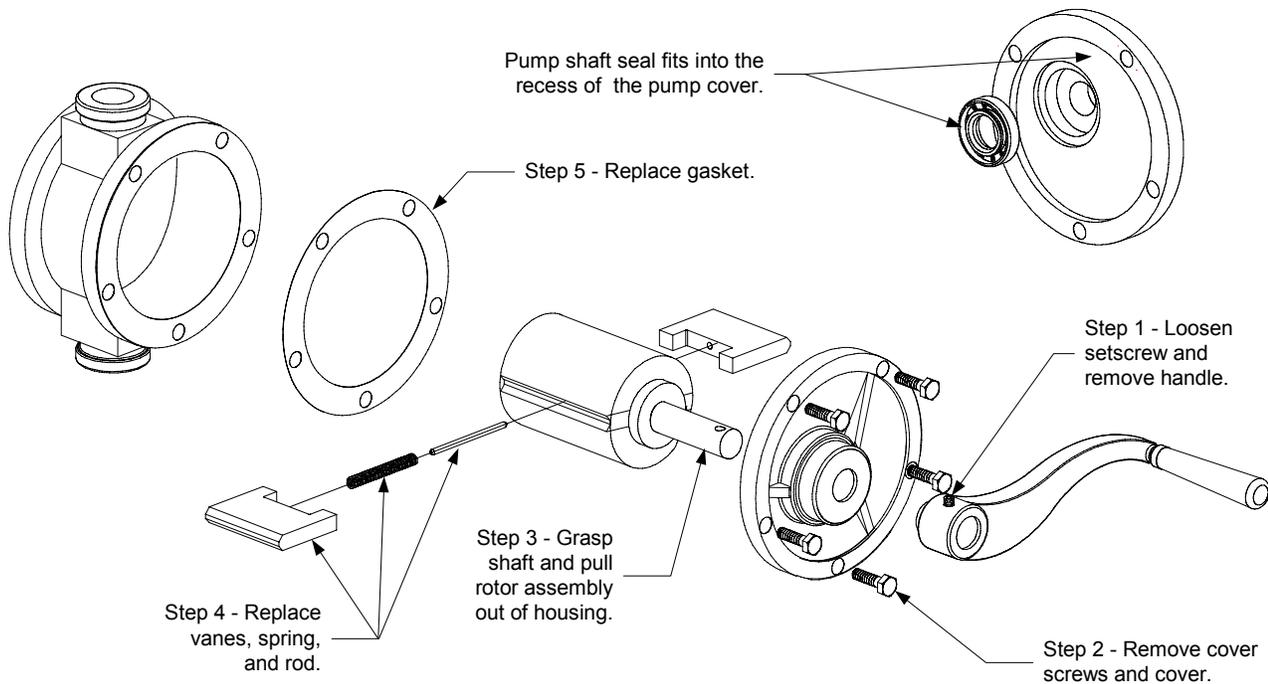
4. Assemble the replacement vanes, spring and rod into the rotor assembly. Compress the vane spring and carefully insert the rotor assembly back into the pump housing.
