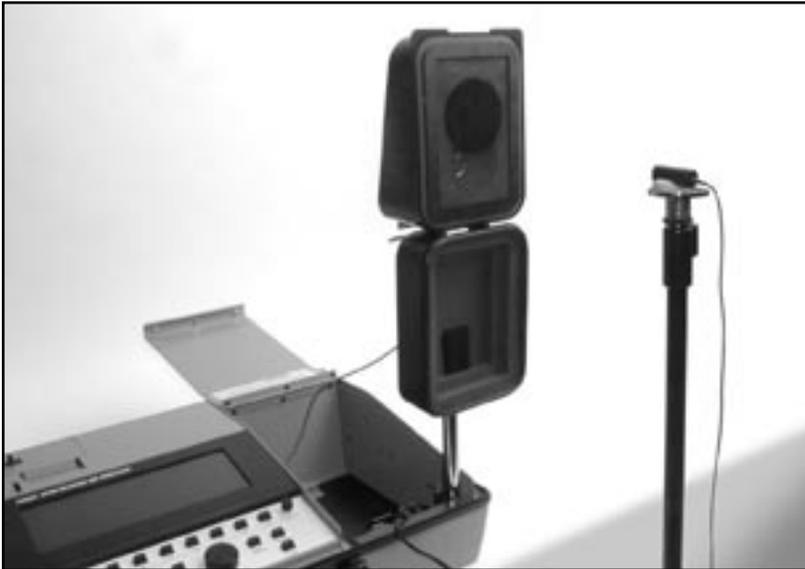
Figure 3.6.1—Preparing for a coupler directional measurement
