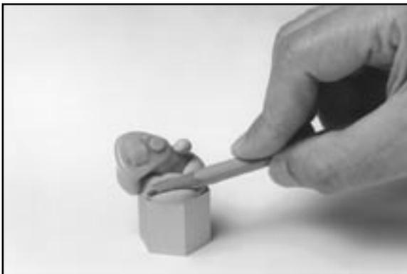
5. Complete the acoustical sealing of the aid to the coupler by using a pencil or finger. You may want to double-check the aid placement through the open end of the coupler at this point.
