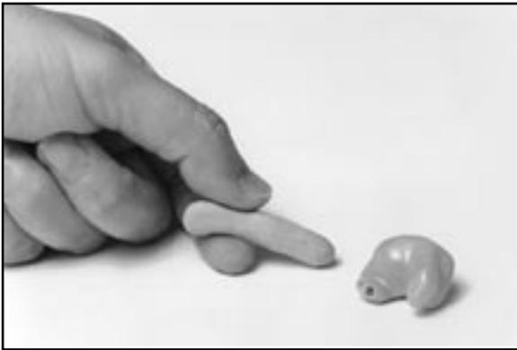
1. Roll some Fun-Tak into a rod long enough to go around the transmitting end of the aid. Modeling clay can also be used, but it doesn't work as well.
