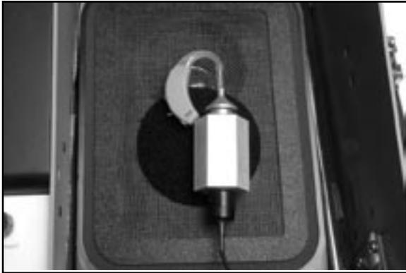
1. Adjust the tone and gain controls of the aid to the desired positions. If desired, insert a battery pill into the aid.
