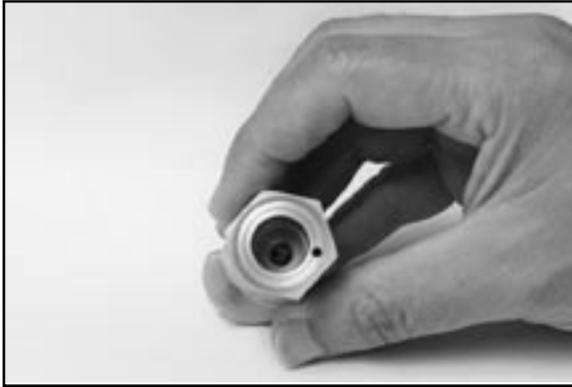
3. Align the sound opening of the aid with the hole at the conical end of the coupler. Look through the open end of the coupler to be sure the sound opening of the aid is clear of obstructions and correctly placed.
