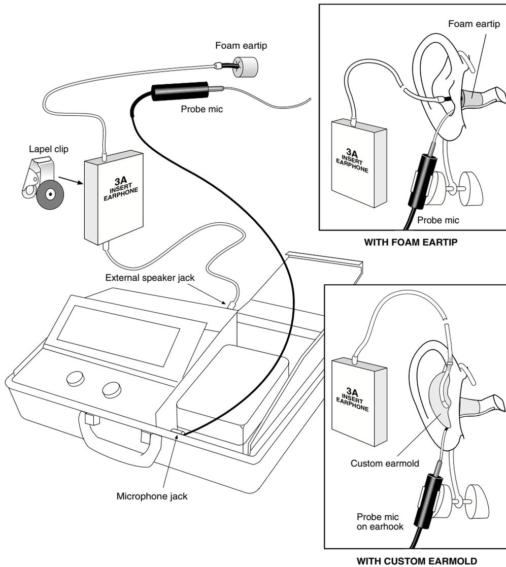
Figure 5.6.1.2A—Setup for real-ear part of the RECD
