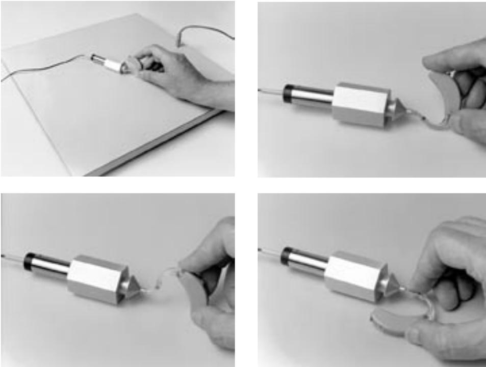
*Figure 7.1B Orienting hearing aid for maximum output*
