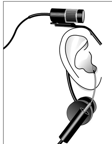
Figure 5.1.2.2—Placing the reference microphone
