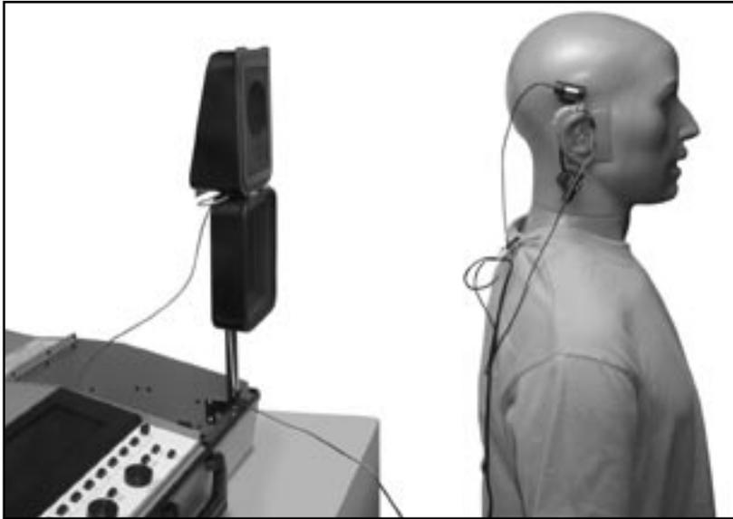
Figure 5.11.1—Reverse measurement positioning for directional test
