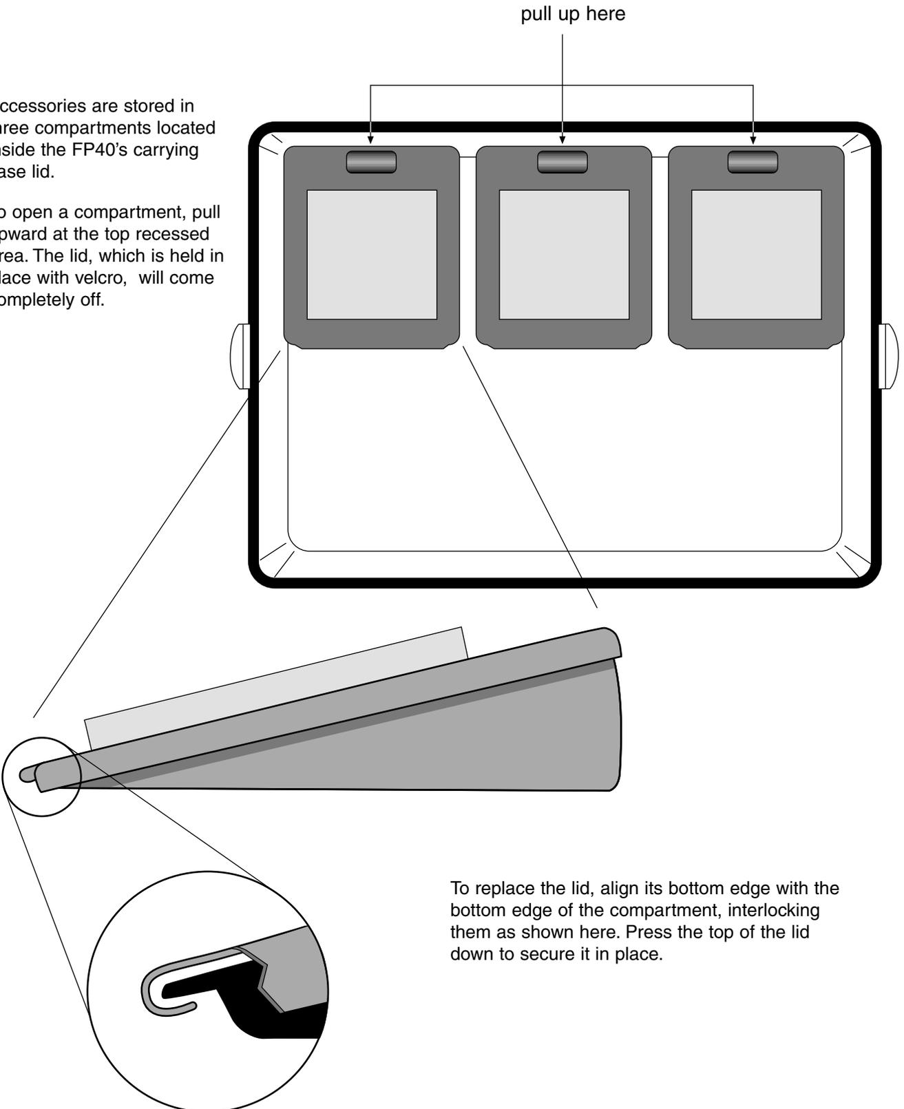
To replace the lid, align its bottom edge with the bottom edge of the compartment, interlocking them as shown here. Press the top of the lid down to secure it in place.
