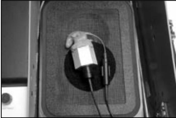
6. Slowly insert the microphone into the coupler. You may feel an initial resistance when the mic reaches the O-ring. Continue to push the microphone until it stops.
