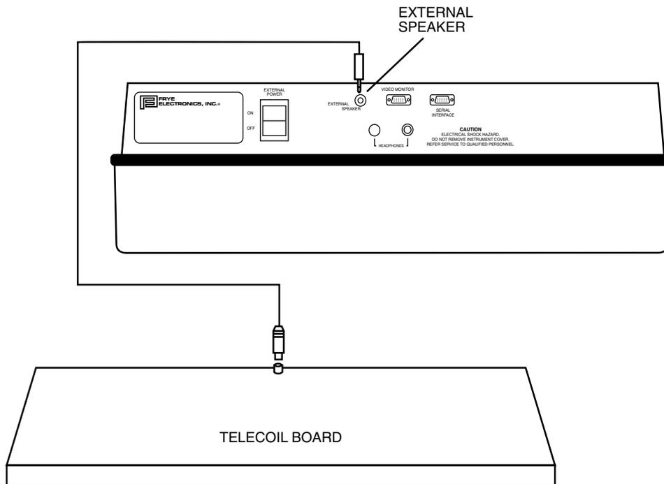
Figure 7.1A Telecoil setup
