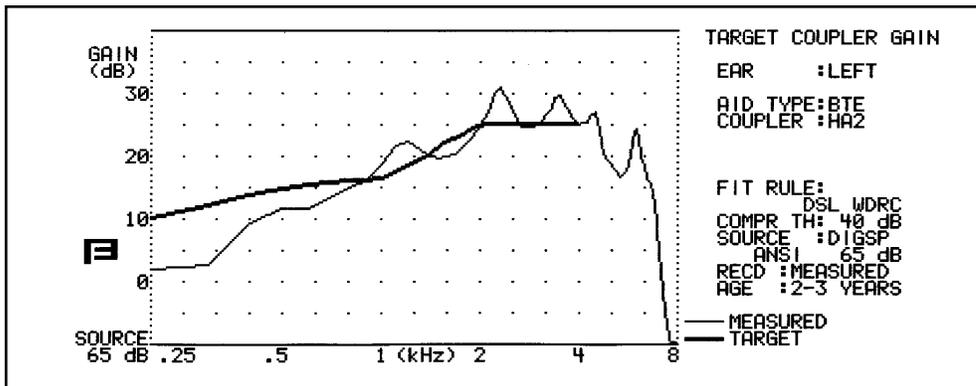
Figure 5.6.2A—Coupler gain measurement with a DSL target
