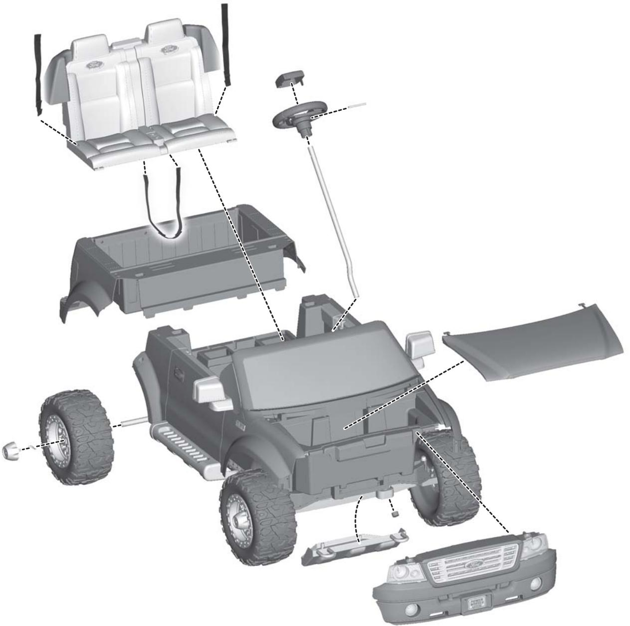
**Note:** Some parts shown are assembled to both sides of the vehicle. Fasteners not shown.
