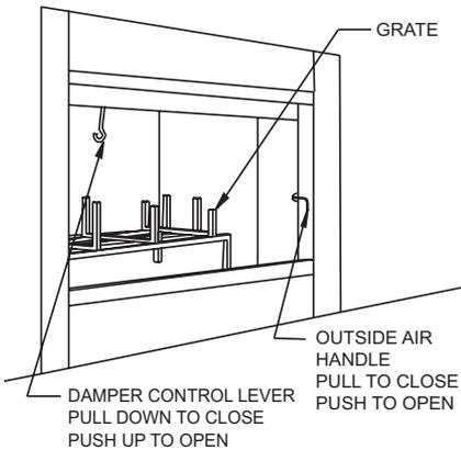
*Figure 32 - Damper Operation*
