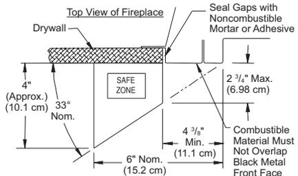
**Figure 12 - Mantel Clearances to Metal Face**
