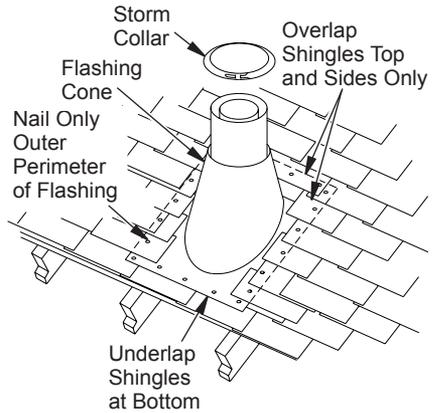
**Figure 24 - Flashing Installation**
