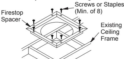
**Figure 20 - Firestop Spacer with Attic Space Above Ceiling**
