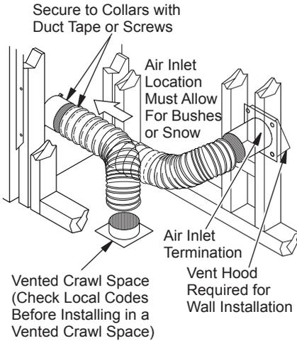
**Figure 13 - Outside Air Kit Installation**
