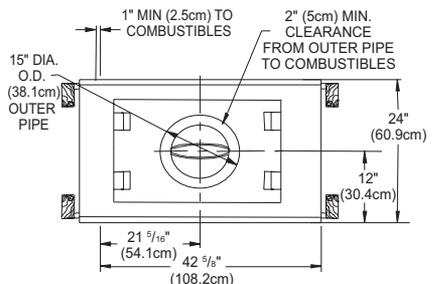
Figure 5 - Framing Clearances
