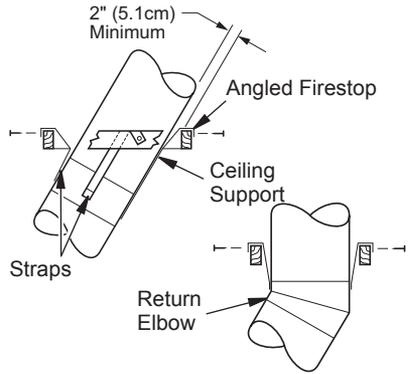
**Figure 17 - Chimney Supports**
