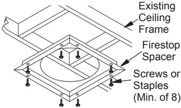
**Figure 19 - Firestop Spacer with Living Space Above Ceiling**
