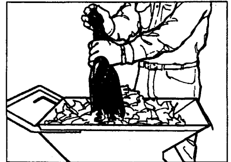
Figure 4-4: Using the leaf tamper to process material into the shredder hopper.
