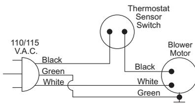
Figure 25 - Wiring Diagram for Blower Accessory
