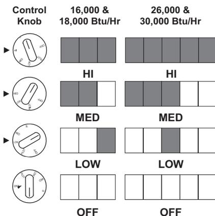
Figure 22 - Burner Patterns for Manual Control Models
