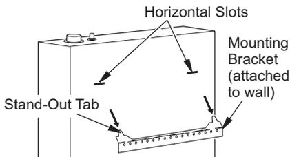
Figure 11 - Mounting Heater onto Mounting Bracket
