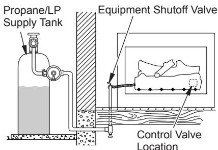
**Figure 17 - Checking Gas Joints for Propane/LP Gas**
