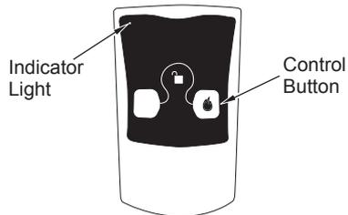
**Figure 26 - On/Off Hand-Held Remote Control Unit**
