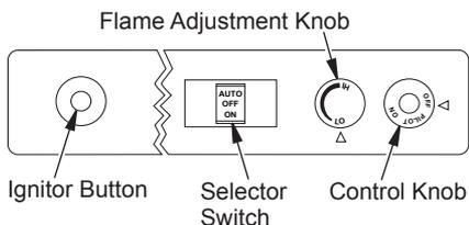
**Figure 22 - Control Knob and Ignitor Button Location (Shown as Supplied, No Control Options)**
