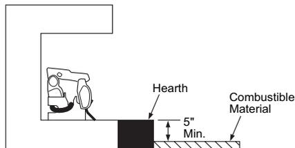
**Figure 9 - Minimum Fireplace Clearances Above Combustible Flooring**
