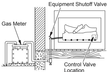
**Figure 16 - Checking Gas Joints for Natural Gas**
