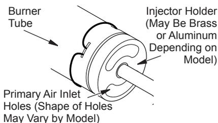
**Figure 32 - Injector Holder On Outlet Burner Tube**
