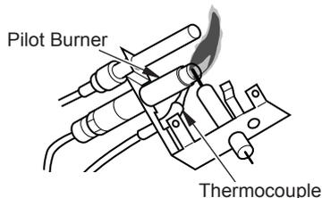
**Figure 29 - Incorrect Pilot Flame Pattern (Propane/LP Pilot Shown)**
