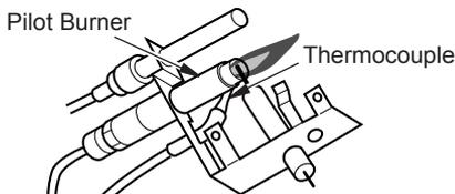
**Figure 28 - Correct Pilot Flame Pattern (Propane/LP Pilot Shown)**
