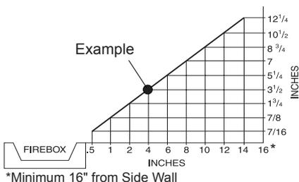
**Figure 4 - Minimum Clearance for Combustible to Wall**
