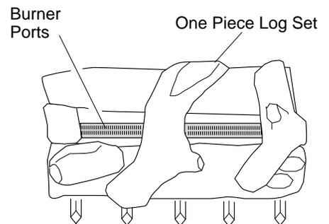
Figure 19 - Installing Heat Majic™ One-Piece Log Set (Top View)
