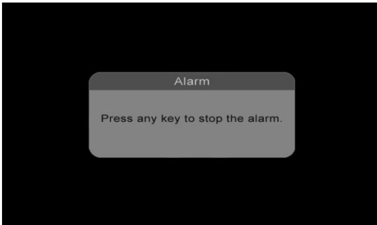
User can press any key to exit the alarm mode and end the alarm tone or it will turn off automatically after 5 minutes of continuous alert.
