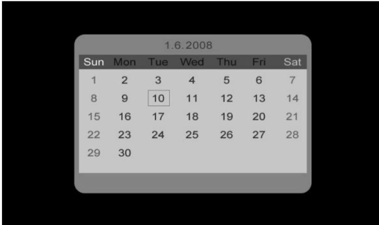
During calendar display screen, you can press ▲ or ▼ buttons to scroll through the month or press ◀ or ▶ button to scroll the year.
