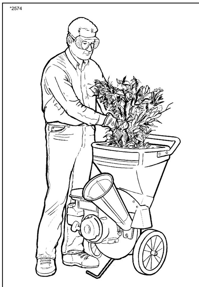
Figure 9. Properly Feeding Longer Materials for Shredding
