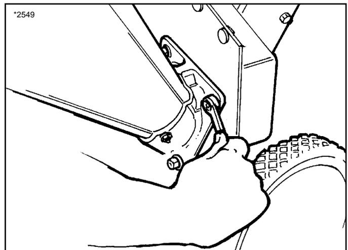
Figure 23. Removing Chipper Cone to Expose Chipping Knives.
