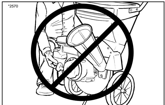
Figure 15. Improper Lifting Of Unit
