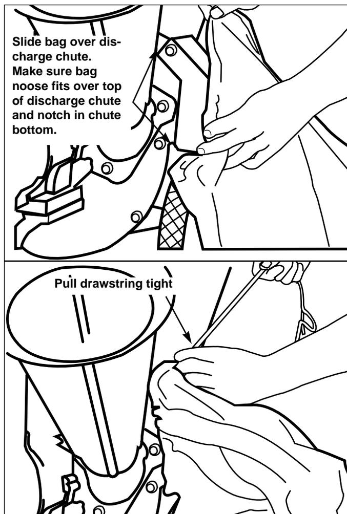
Figure 5B. Discharge Bag Installation-European model
