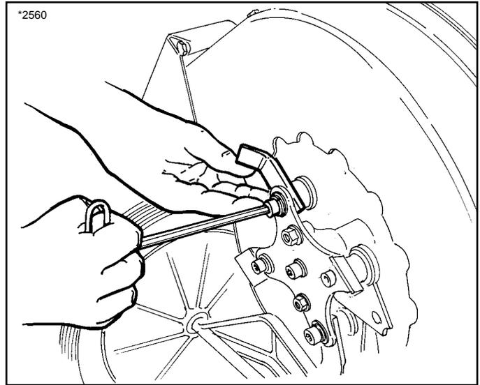
Figure 21. Reassembling Shredder Hammer
