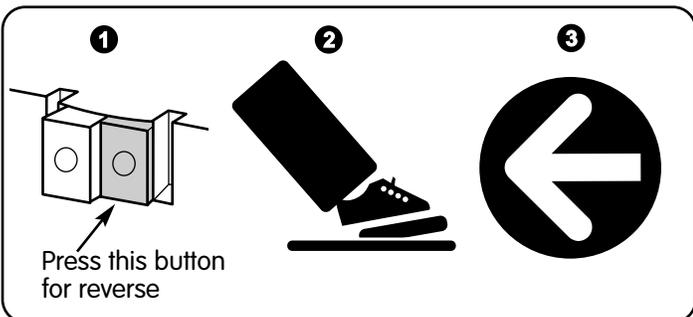
**IMPORTANT!** To avoid damaging the motors and gears, be sure to stop the vehicle before switching from forward to reverse.
