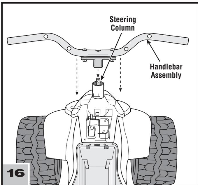
**Hint:** You may want the help of another adult to support the steering column near the steering linkage while assembling the handlebar to the vehicle.
