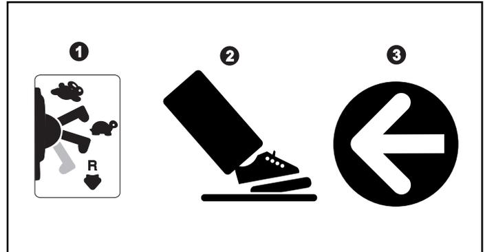
**Please Note: To avoid damaging the motors and gears, stop the vehicle before shifting from forward to reverse (
