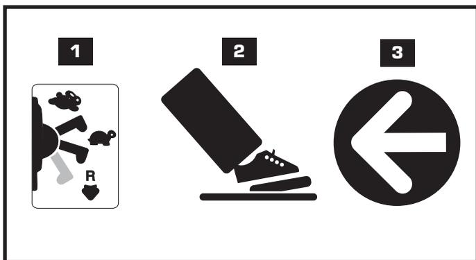
**IMPORTANT!** To avoid damaging the motors and gears, stop the vehicle before shifting from forward to reverse
