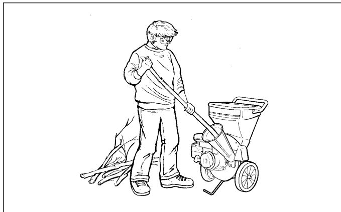
Figure 9. Chipping of Tree Limbs
