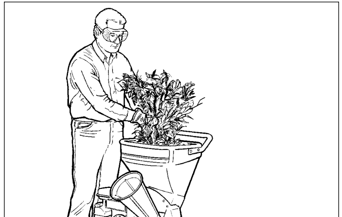
Figure 13. Feeding Brush and Longer Shreddables
