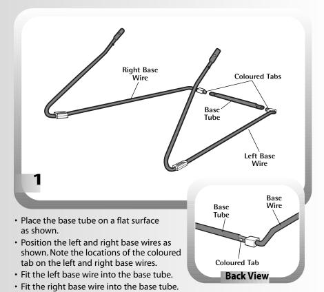
· Make sure both coloured tabs on the base wires are visible through
