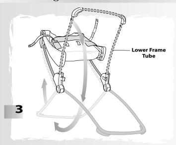
• Rotate the lower frame tube around to the top of frame, as shown.
