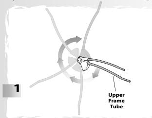
• Rotate the upper frame tube until it "snaps" into an upright position, as shown.
