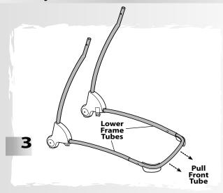
• Pull the front tube to be sure it is secure to each lower frame tube.
