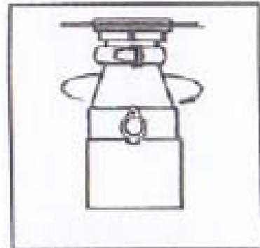
3. Slide the waste pipe flange on to the waste pipe.
