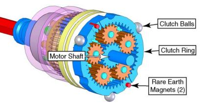
Another feature of the C12 gearbox is the integral shaft-lock to assist in bit changing. The motor can rotate the drill chuck, but the drill chuck cannot
