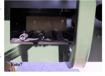
of the hopper (191) by unbolting the four nuts (118) so that you can clean the apron conveyor (145) and the driven roller (185) through the inspection overlay of the hopper (picture 7). Please make sure that the apron conveyor is not too stretched (there should be a 3/4 cm subsidence when pressing the upper part of the apron conveyor itself at around 15 cm from its beginning). If so, loosen it by using the threaded bars (187).
