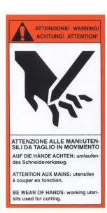
This sticker informs that the protections of the cutting heads and the hammers have been designed to prevent the operator, who stands in front of the machine, from touching them. However, especially from the front material discharge, he could get to the blades, if he leaned forward. Should it be necessary for the operator to lean forward, please make sure to take all the necessary precautions, like switching the machine off or wearing your protection gloves.
