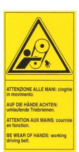
This sticker informs the operator that under the protection devices there are some driving-belts working. It is therefore absolutely forbidden to put your hands in the spaces the manufacturer left open for the machine to cool off. It is also forbidden to use the machine without the protection devices.
