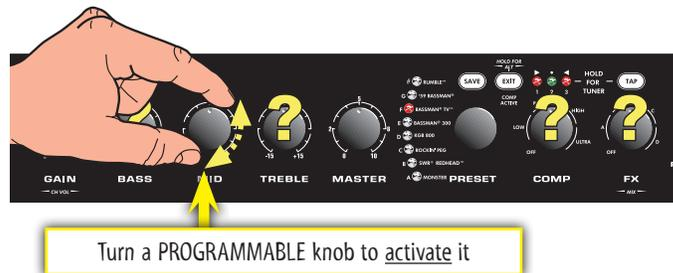
You may hear a big change in volume or tone when you first turn a programmable knob if there happened to be a large difference between the knob's starting position and the stored preset setting. For example, if the VOLUME knob is pointing to "8" but the stored preset VOLUME setting is "2," the volume level will jump from "2" to "8" when you start turning the VOLUME knob because the VOLUME knob is now instantly active at "8."
