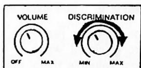
You can set DISCRIMINATION to minimum (fully counterclockwise), to maximum (fully clockwise), or anywhere in between. As you set DISCRIMINATION to higher levels, the detector first does not detect small pieces of silver paper, then thick foil, and finally metal objects like pull tabs from aluminum cans.
