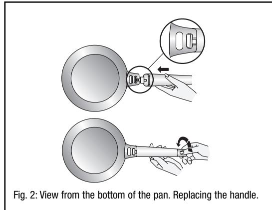
Slide the protruding rectangular metal end of the handle into the notch on the end of the body of your piece of cookware.
