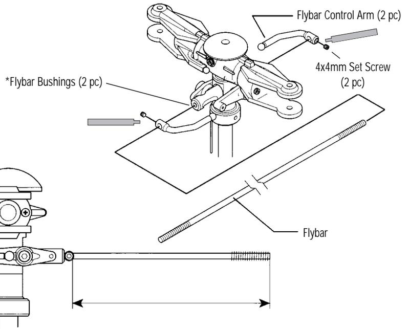
**Note:** Center the Flybar in the Seesaw Shaft before securing the two Flybar Control Arms.
