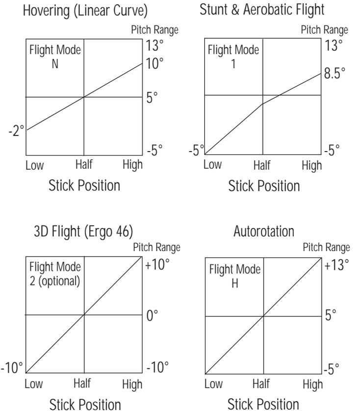
**Note:** When using the "B" style double link set for 3D flight, the maximum pitch range is altered to +10° - -10°, reducing the + pitch range for autorotations.
