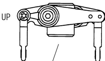
Long portion of mixing base flange must face downward.
