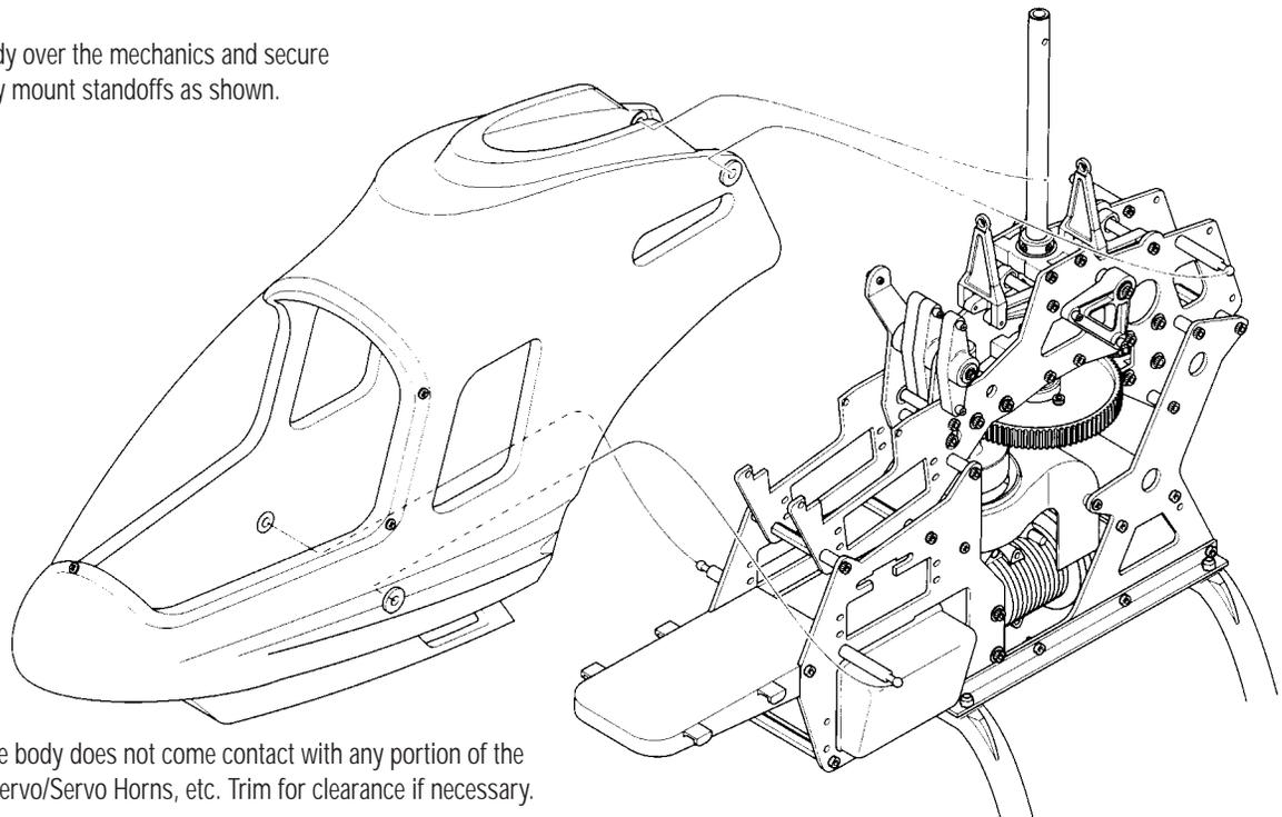
Check to insure that the body does not come contact with any portion of the Main Frame, Muffler, Servo/Servo Horns, etc. Trim for clearance if necessary.
