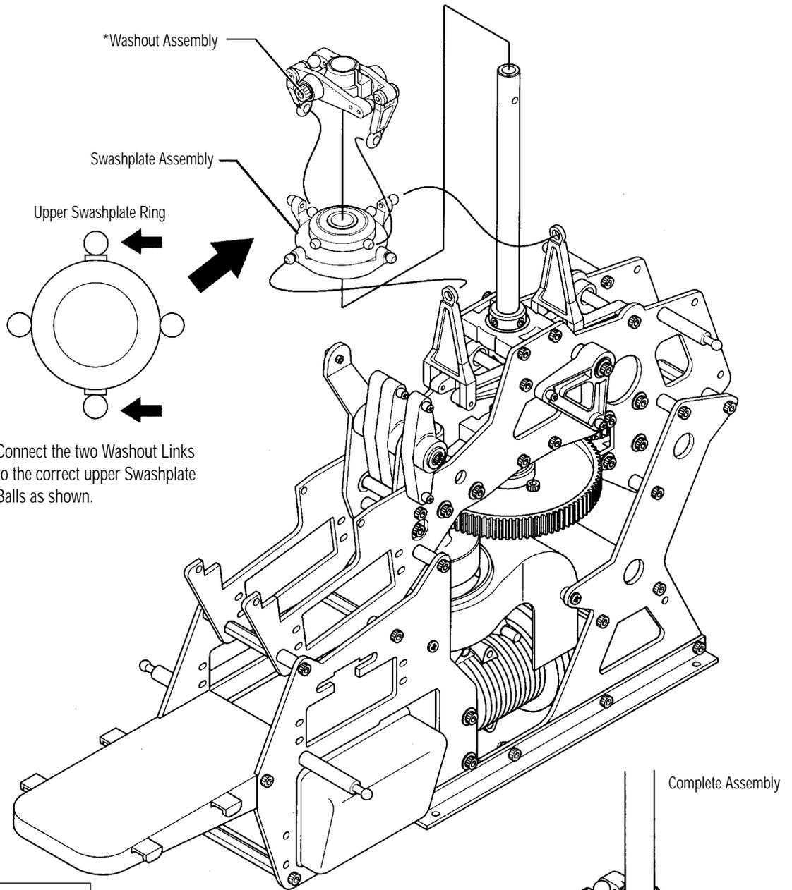
Connect the two Washout Links to the correct upper Swashplate Balls as shown.
