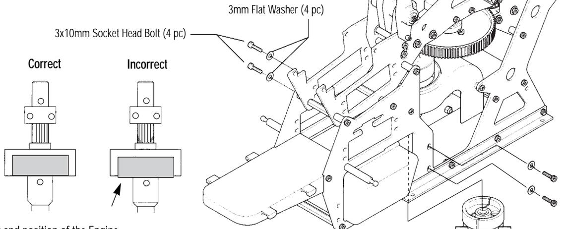
Adjust the height and position of the Engine as shown so the bottom of the Clutch Assembly is flush with the bottom of the Clutch Bell. Also check to insure that the Engine and Clutch Bell are parallel.
