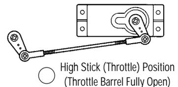
\*To avoid differential throttle travel, make certain both the throttle arm and the servo horn are positioned as shown in the above diagrams.
