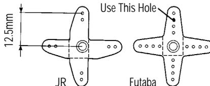
Be sure to remove the excess Servo Horn Arms as shown. Secure the Servo Horn using the Servo Horn Screw.
