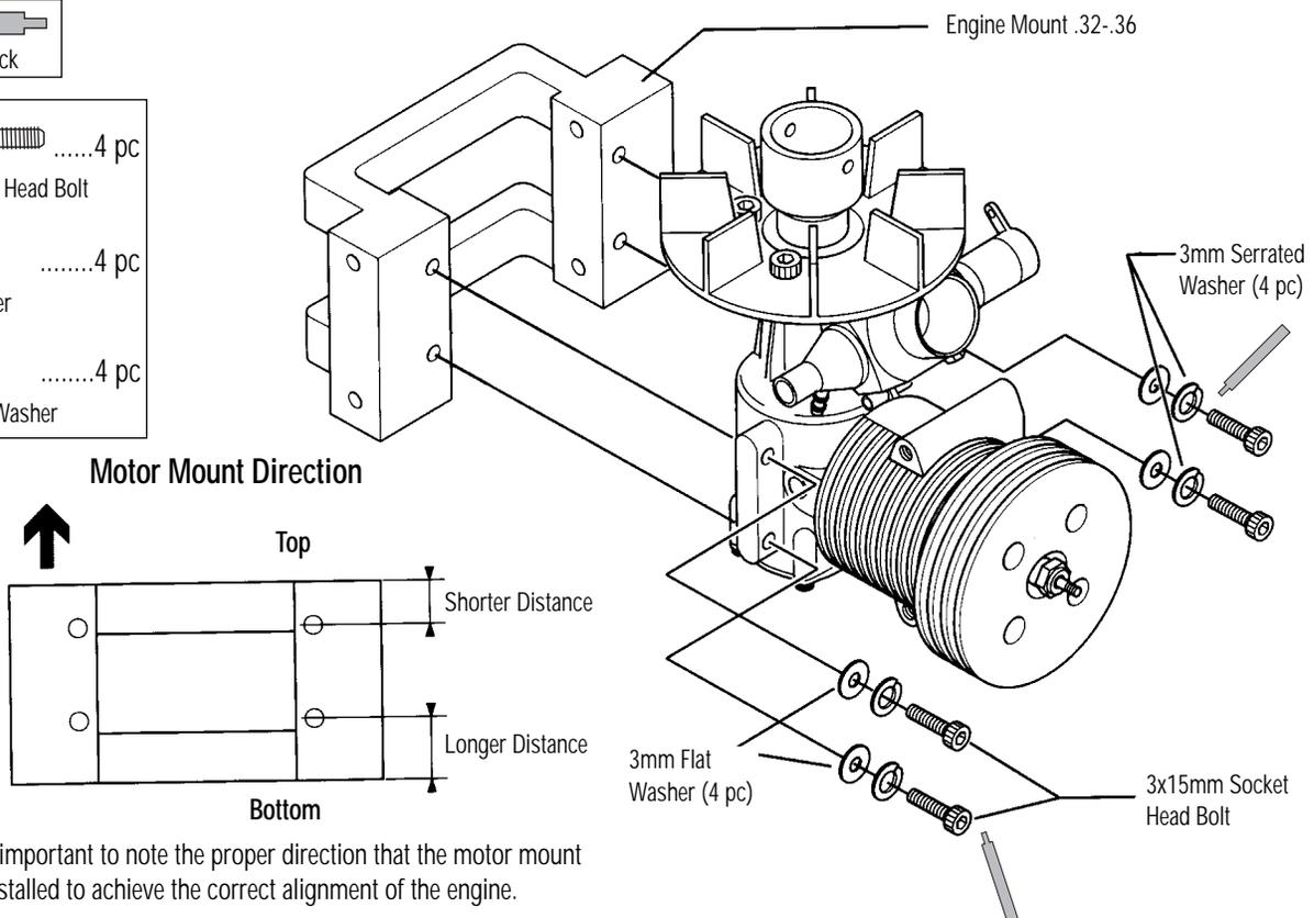
It is important to note the proper direction that the motor mount is installed to achieve the correct alignment of the engine.
