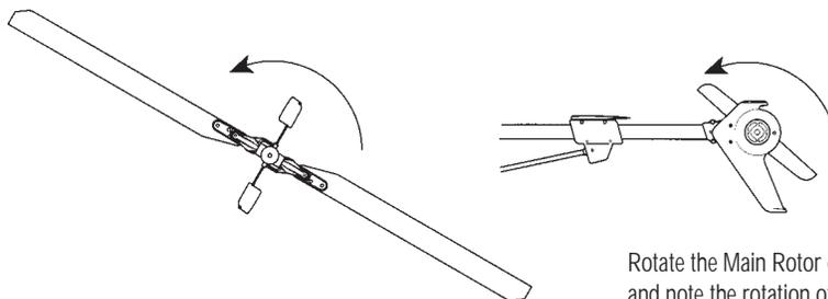
Rotate the Main Rotor counter clockwise (backward) and note the rotation of the Tail Rotor.
