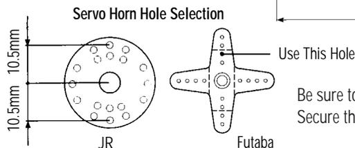
Be sure to remove the excess Servo Horn Arms as shown. Secure the Servo Horn using the Servo Horn Screw.
