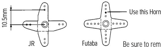
Be sure to remove the excess Servo Horn Arms as shown. Secure the Servo Horn using the Servo Horn Screw.
