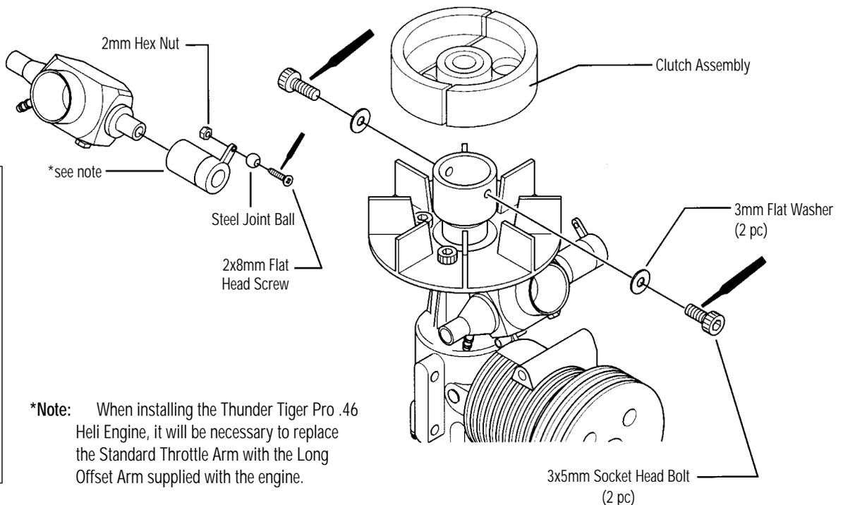
**\*Note:** When installing the Thunder Tiger Pro .46 Heli Engine, it will be necessary to replace the Standard Throttle Arm with the Long Offset Arm supplied with the engine.
