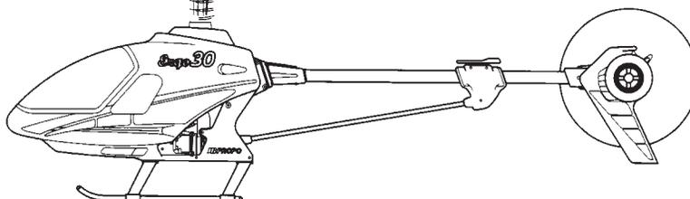
**Caution:** Be sure to maintain a safe distance from the helicopter (15 to 20 feet) when tracking main rotor blades.
