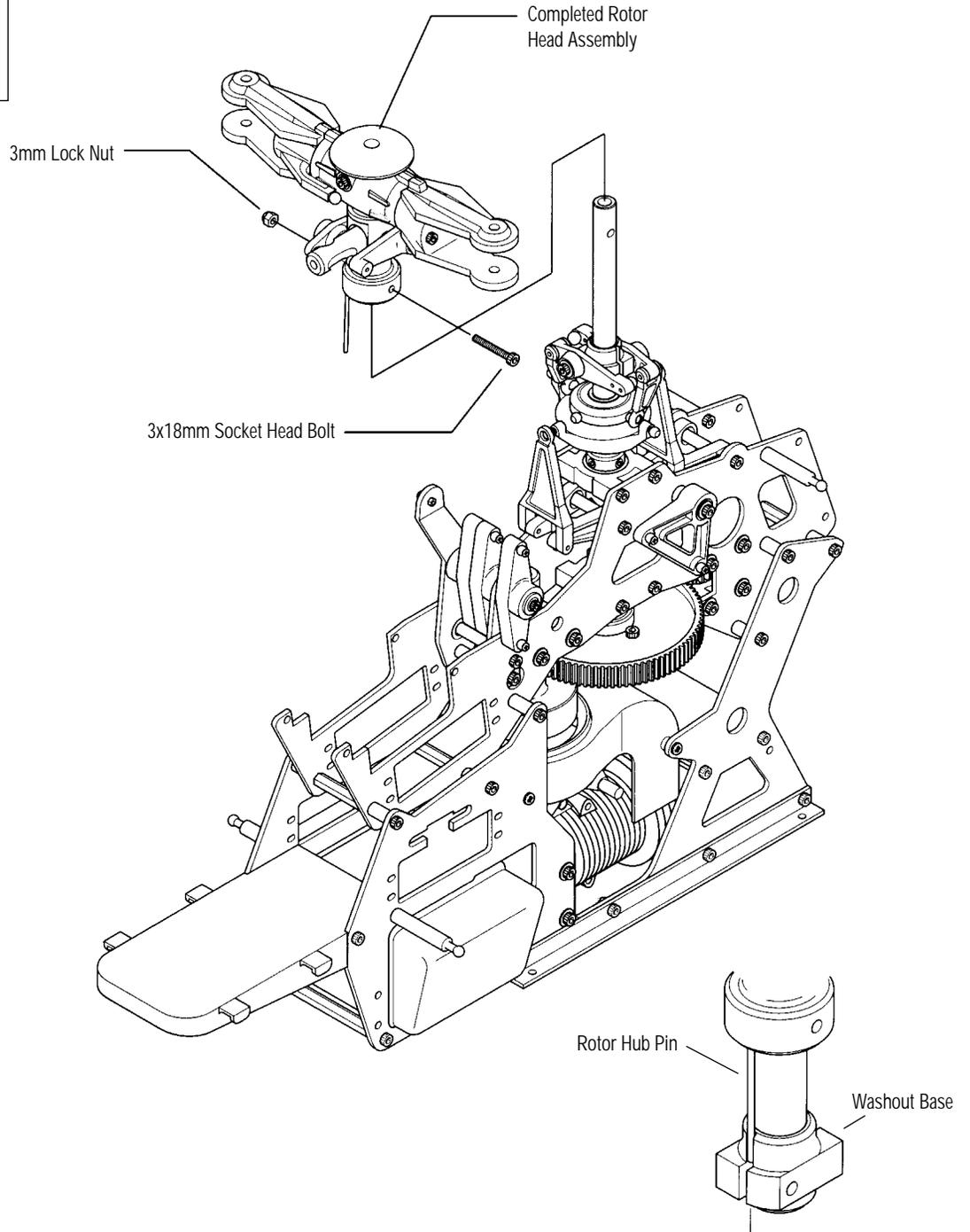
**Note:** Be sure to engage the Phase Adjusting Ring into the Washout Base Groove before securing the Rotor Head Assembly in place.
