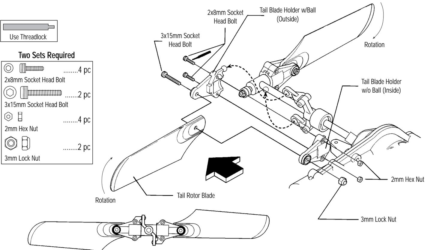
\* Be sure to note direction of Tail Rotor Blades during assembly.
