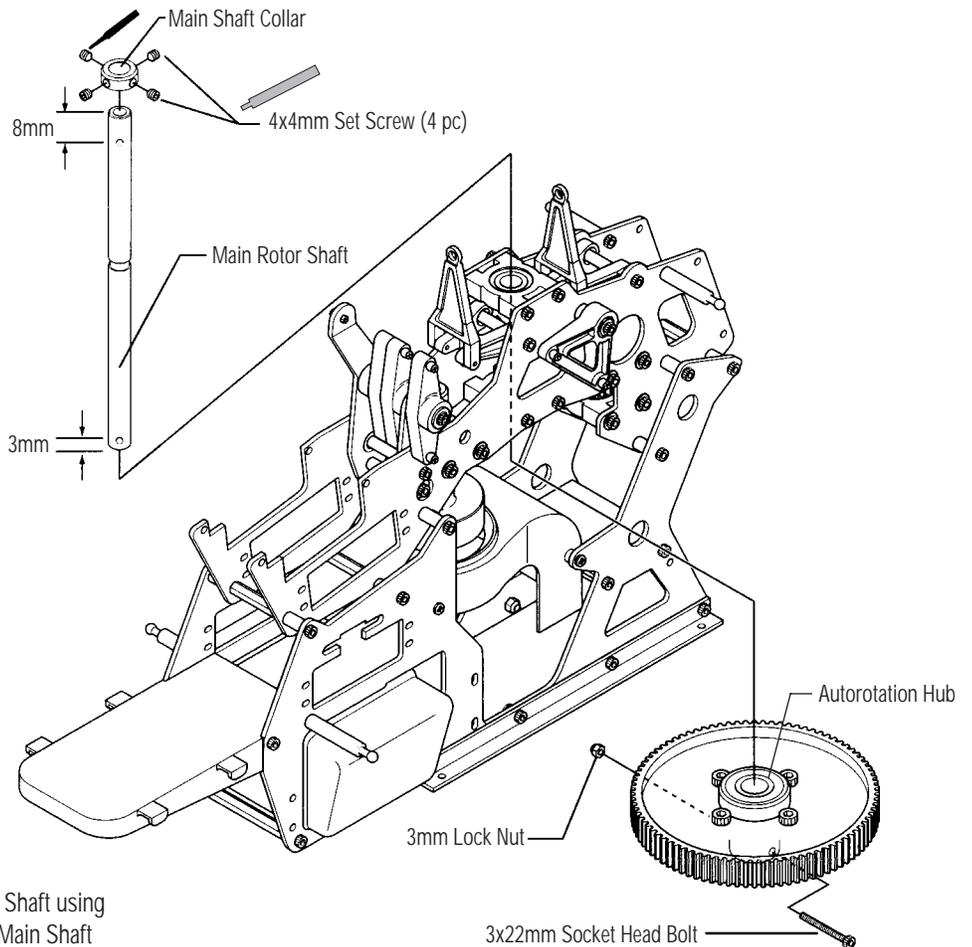
1. Secure the Autorotation Hub to the Main Rotor Shaft using the 3x22mm Socket Head Bolt. Next, slide the Main Shaft Collar onto the Main Rotor Shaft. While pulling upward on the Main Rotor Shaft, secure the Main Shaft Collar to the Main Rotor Shaft using the four 4x4mm Set Screws.
