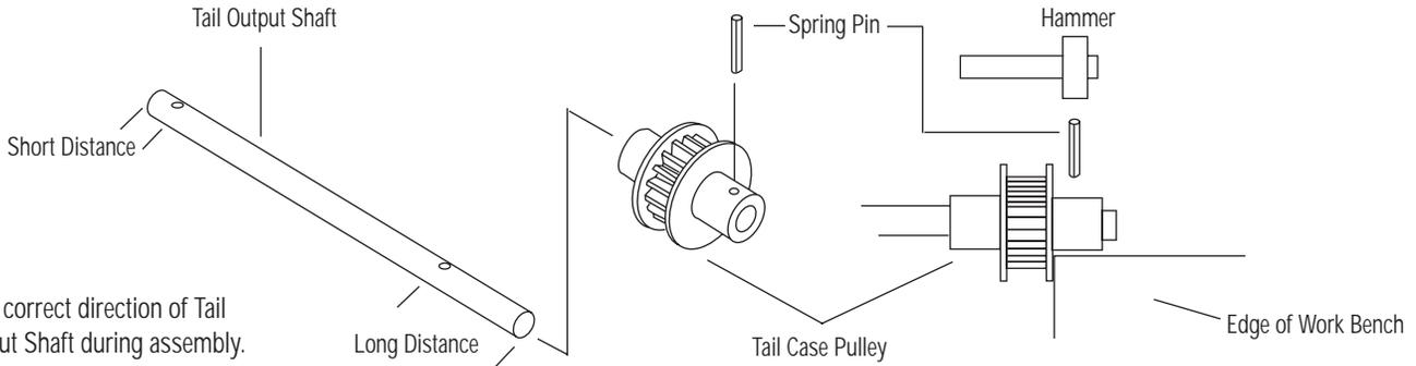
Note correct direction of Tail Output Shaft during assembly.
