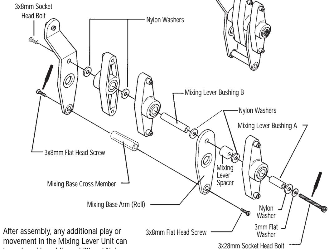
After assembly, any additional play or movement in the Mixing Lever Unit can be reduced by adding additional Nylon Washers as needed.
