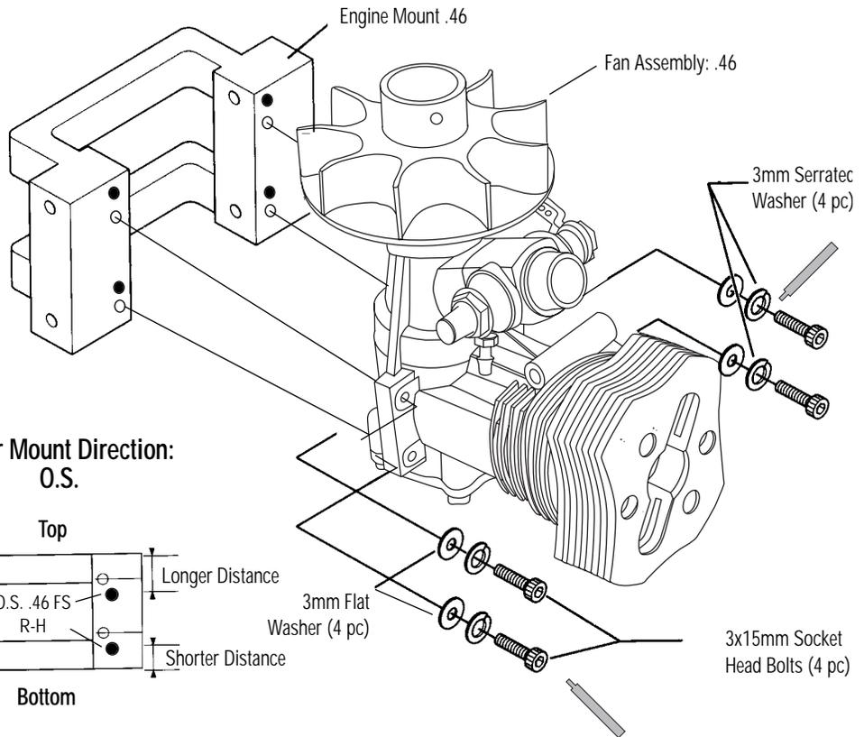
It is important to note the proper direction that the Motor Mount is installed to achieve the correct alignment of the engine.
