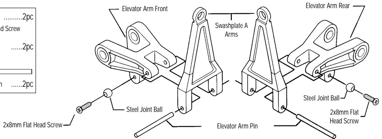
**Caution:** Be sure to note correct Swashplate A Arm installation direction.
